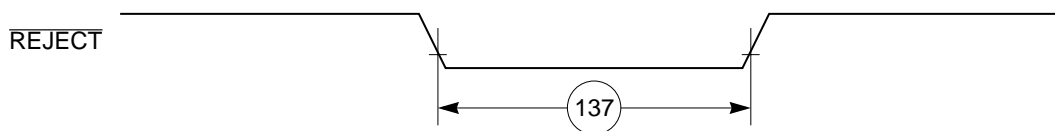
Figure 11-61. CAM Interface REJECT Timing Diagram
