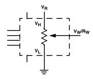
THREE-TERMINAL POTENTIOMETER; VARIABLE VOLTAGE DIVIDER
