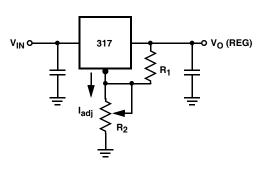
$V_O (REG) = 1.25V (1+R_2/R_1)+ladj R_2$
