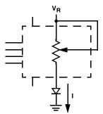
TWO-TERMINAL VARIABLE RESISTOR; VARIABLE CURRENT
