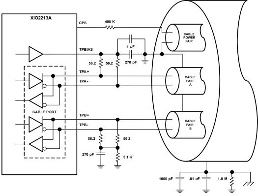
The IEEE Std 1394-1995 calls for a 250-pF capacitor, which is a nonstandard component value. A 270-pF capacitor is recommended.
