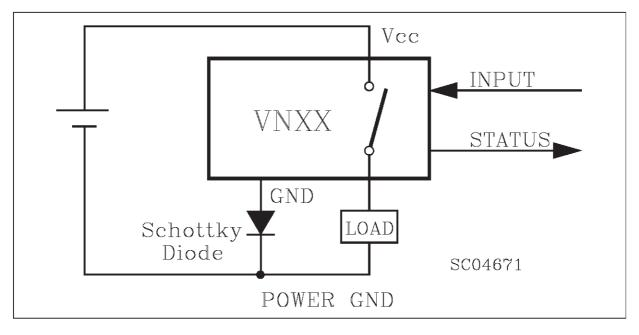
Figure 3: Typical Application Circuit With A Schottky Diode For Reverse Supply Protection
