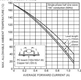
Max. allowable lead temperature (Resistive or inductive load)
