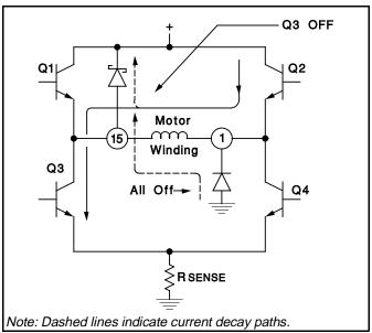
Figure 7: Simplified Schematic of Output Stage
