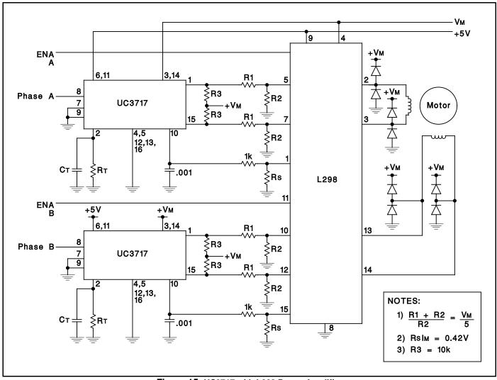
Figure 15: UC3717 with L298 Power Amplifier
