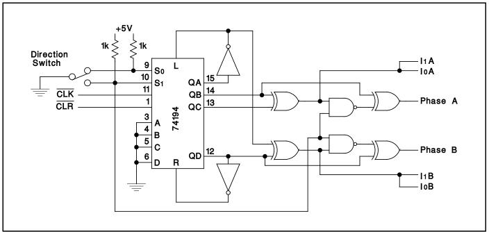
Figure 14: Half-Step, Bidirectional Drive Logic
