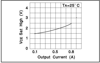
Figure 2: Typical Source Saturation Voltage vs Output Current
