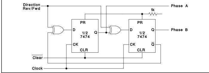
Figure 13: Full Step Bidirectional Two Phase Drive Logic
