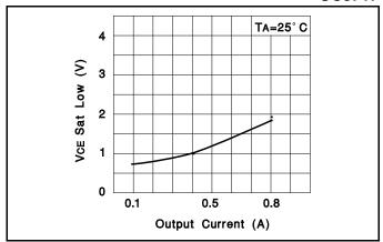
Figure 3: Typical Sink Saturation Voltage vs Output Current
