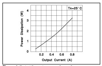
Figure 4: Typical Power Losses vs Output Current
