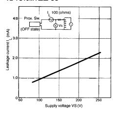
Note: Even when the proximity sensor is in the OFF state, a very small amount of current flows to operate the internal circuit of the sensor. Because of this leakage current, a small voltage is generated in the load, which may occasionally result in improper resetting of the load. Before using the proximity sensor, confirm that this voltage is less than the release voltage value of the load.
