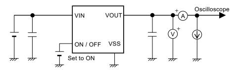
Figure 16 Test Circuit 7
