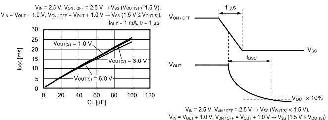
Figure 35 S-19243xxxA Series A / B type (with discharge shunt function)
