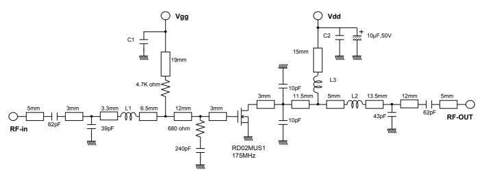
L1:Enameled wire 5 Turns,D:0.43mm,2.46mmm O.D L2:Enameled wire 3 Turns,D:0.43mm,2.46mmm O.D L3:Enameled wire 9 Turns,D:0.43mm,2.46mmm O.D C1,C2:1000pF,0.0022µF in parallel Note:Board material PTFE substrate Micro strip line width=2.2mm/50 ohm,er:2.7,t=0.8mm
