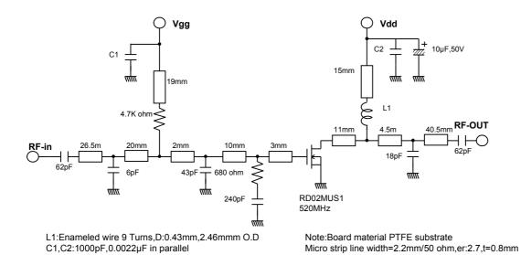
RoHS Compliance, Silicon MOSFET Power Transistor 175MHz, 520MHz, 2W
