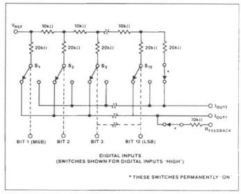
FIGURE 1: Simplified DAC Circuit
