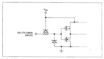
FIGURE 2: Digital Input Protection
