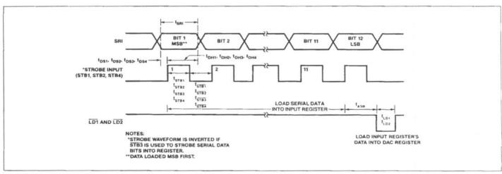
FIGURE 6: Timing Diagram
