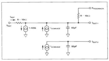
FIGURE 4: PM-7543 Equivalent Circuit (All Digital Inputs HIGH)
