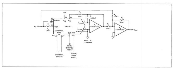
FIGURE 9: Bipolar Operation (4-Quadrant, Offset Binary)
