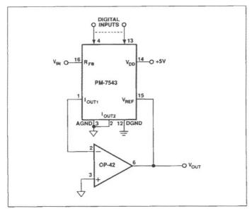
FIGURE 10: Analog/Digital Divider
