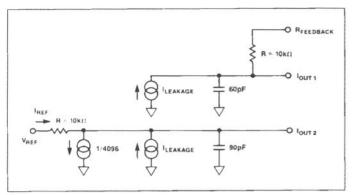
FIGURE 3: PM-7543 Equivalent Circuit (All Inputs LOW)
