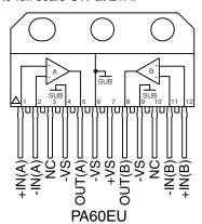
FIGURE 3. External connections
