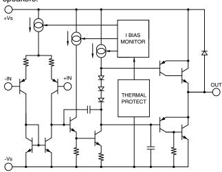
FIGURE 1. Equivalent schematic (one channel)
