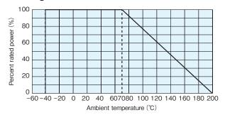
For resistors operated at the ambient temperature of 70°C or higher, the power rating shall be derated in accordance with the above derating curve.
