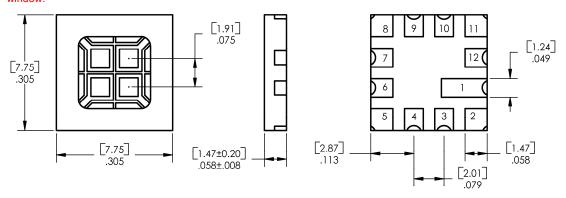
TOLERANCE IS  $\pm .005$  [ 0.13 ] DIMENSIONS ARE IN INCHES AND [MILLIMETERS].
