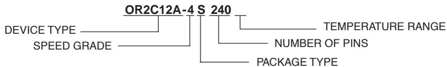
OR2C12A, -4 speed grade, 240-pin shrink quad flat pack, commercial temperature.
