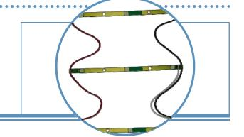
The **OPA775 and OPA776** are designed for areas where lighting intensity and reliability are essential. The light beam angle of 120° is ideal for illuminating small and medium size areas while requiring minimal space. The devices are mounted on an FR-4 PC Board for ease of use with an easy to use IDC connector interface.
