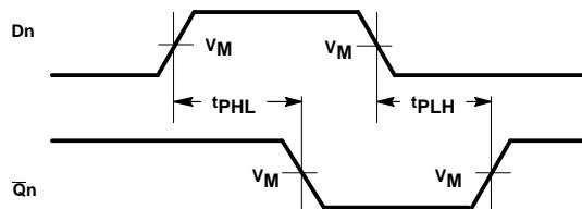
Waveform 1. Propagation delay for inverting outputs
