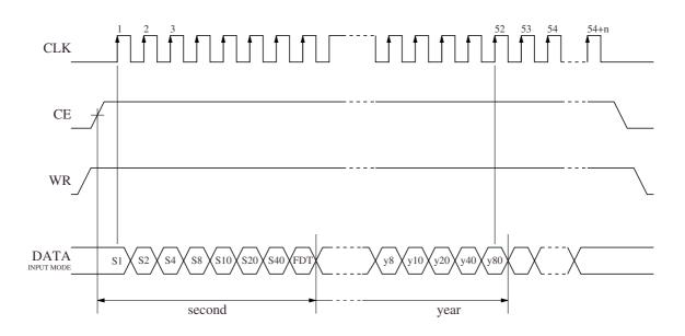
Data is input when WR is HIGH and CE is HIGH.
