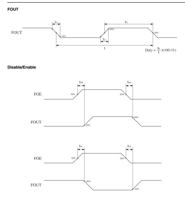
Note that FOE and FSEL do not have chatter elimination circuits. Consequently, switching either FOE or FSEL during 32kHz mode operation may generate chatter noise on the FOUT output. Also, note that the 1Hz and 32kHz oscillators are not synchronized to each other, so switching intervals shortens the duty cycle. Accordingly, a wait time ( $\geq$  chattering time + output frequency period) should be incorporated when switching intervals.
