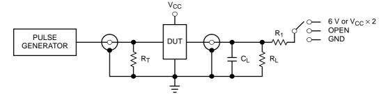
Figure 4. Test Circuit
