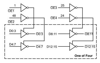
Figure 2. Logic Diagram
