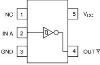
Figure 1. Pinout (Top View)
