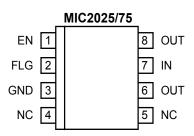
8-Lead SOIC (BM) 8-Lead MSOP (BMM)
