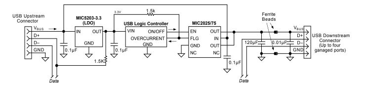
Figure 6. USB Bus-Powered Hub
