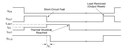
Figure 1. MIC2075-2 Timing: Output Reset by Removing Load
