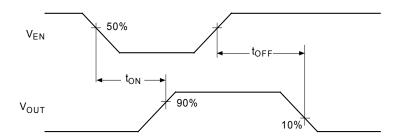
Active-Low Switch Delay Times (MIC20x5-2)
