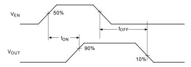
Active-High Switch Delay Times (MIC20x5-1)
