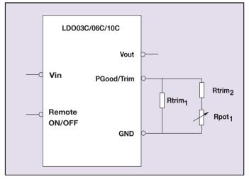
Figure 12 - Output Voltage - with Potentiometer
