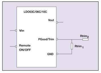
Figure 11 - Output Voltage Trim - with Voltage Source
