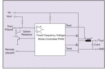
Figure 1 - Electrical Block Diagram
