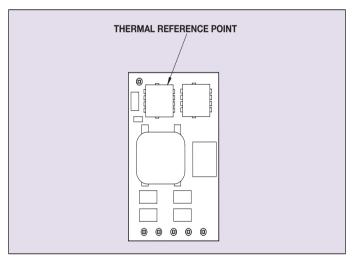
Figure 9 - LDO06C/10C Thermal Reference Point Location Converters
