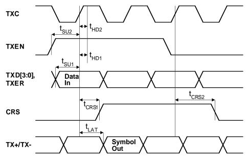
Figure 5. 100BASE-T MII Transmit Timing
