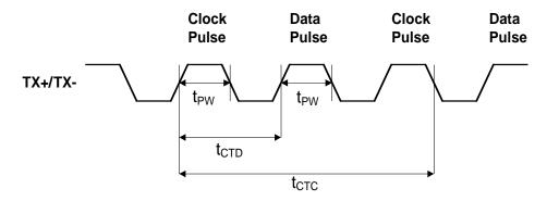
Figure 7. Auto-Negotiation/Fast Link Pulse Timing
