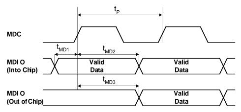
Figure 8. Serial Management Interface Timing
