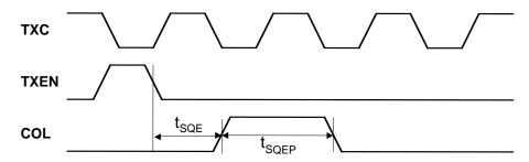
Figure 4. 10BASE-T MII Transmit Timing
