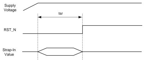
Figure 9. Reset Timing
