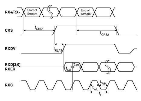
Figure 6. 100BASE-T MII Receive Timing
