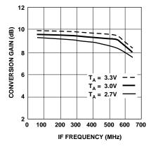
Figure 11. Conversion Gain vs. Frequency and Supply Voltage.
