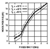
Figure 2. Moise Figure (into 50  $\Omega$ ) vs. Frequency and Temperature.
