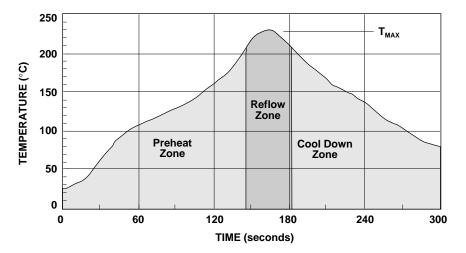
Figure 36. Surface Mount Assembly Profile.
