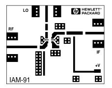
Figure 28. PCB Layout.
