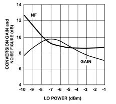
Figure 13. Available Conversion Gain and Noise Figure vs. LO Drive Power.
