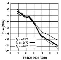
Figure 3. OutputPower (@ 1 dB Comparison) vs. Frequency and Temperature.
