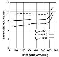
Figure 10. SSB Noise Figure vs. Frequency and Temperature.
