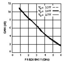
Figure 4. Available Conversion Gain vs. Frequency and Watage.
