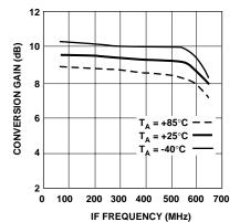
Figure 12. Conversion Gain vs. Frequency and Temperature.
