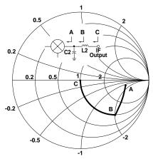
Figure 31. IF Input Impedance Match.
