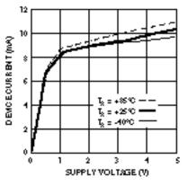
Figure 6. Device Current w. Supply Writage and Temperature.
