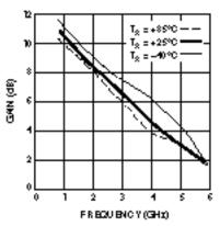
Figure 1. Available Conversion Gain vs. Frequency and Temperature.
