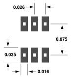
Figure 35. PCB Pad Layout (dimensions in inches).
