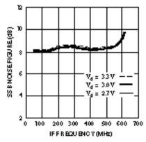
Figure 9. 33B Moise Figure vs. Frequency and Supply Voltage.
