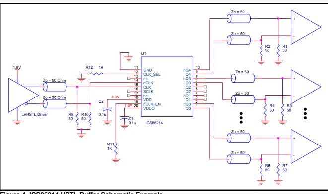
Figure 4. ICS85214 HSTL Buffer Schematic Example
