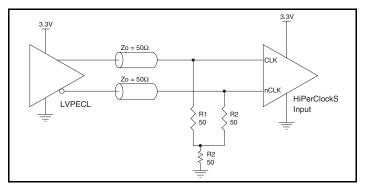
Figure 3B. HiPerClockS CLK/CLK Input Driven by a 3.3V LVPECL Driver
