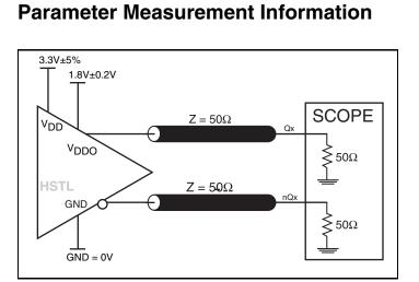
3.3V/1.8V Output Load AC Test Circuit
