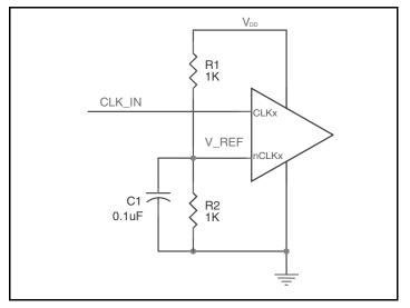
Figure 2. Single-Ended Signal Driving Differential Input
