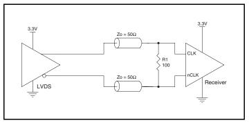
Figure 3D. HiPerClockS CLK/CLK Input Driven by a 3.3V LVDS Driver
