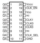
ICS85214 20-Lead TSSOP 6.5mm x 4.4mm x 0.925mm package body G Package Top View
