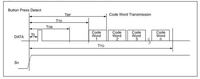
TABLE 7-2: POWER-UP AND TRANSMIT TIMING<sup>(2)</sup>
