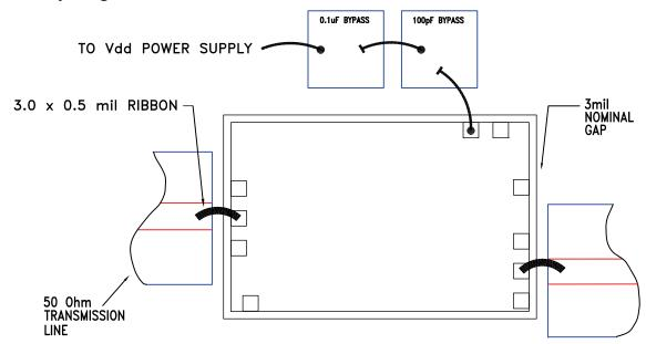
Note 1: Bypass caps should be 100 pF (approximately) ceramic (single-layer) placed no farther than 30 mils from the amplifier.
