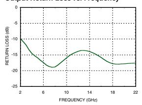
Note: Measured Performance Characteristics (Typical Performance at  $25^{\circ}$ C) Vd= 2.0 V, Id = 55 mA
