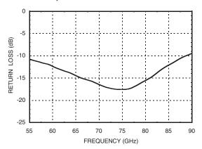
Note 1: Measured Performance Characteristics (Typical Performance at 25°C) Test data is taken with probes on RFIN and RFOUT1 with RFOUT2 left open.
