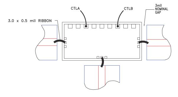
Note 1: Bypass caps should be 100 pF (approximately) ceramic (single-layer) placed no farther than 30 mils from the switch.
