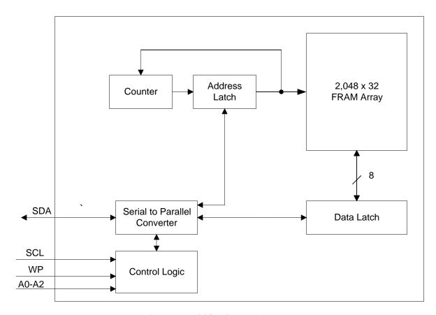
Figure 1. FM24CL64 Block Diagram
