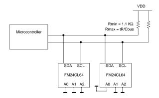
**Figure 2. Typical System Configuration**
