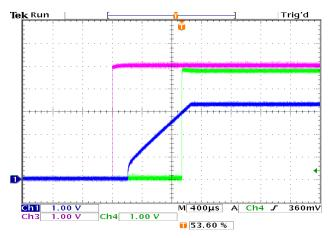
Start up waveforms V<sub>IN</sub>=5.0V, V<sub>OUT</sub>=3.3V, C<sub>SS</sub>=15nF, Ch 1 = V<sub>OUT</sub>, Ch 3 = ENABLE, Ch 4 = POK.
