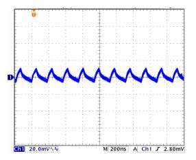
Ripple Voltage, 5.0V<sub>IN</sub>/1.2V<sub>OUT</sub>,  $I_{OUT}$ =6A,  $C_{OUT}$  = 3x22uF.
