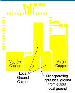
Figure 5. Layout of power and ground copper.
