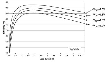
Efficiency vs. Load,  $V_{IN} = 3.3V$ .; Load = 0-6A.
