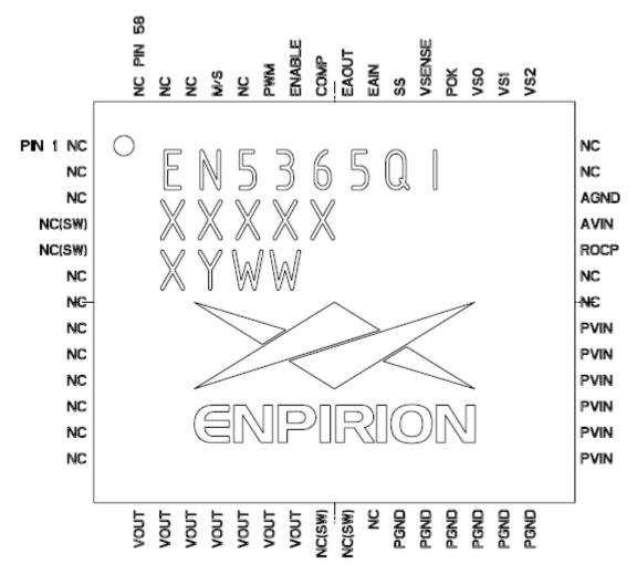
Figure 2. Pin Diagram, top view.
