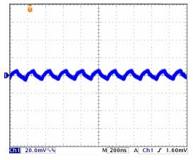
$\label{eq:linear} \begin{array}{l} \mbox{Ripple Voltage, } 3.3 \mbox{V}_{\mbox{IN}} / 1.2 \mbox{V}_{\mbox{OUT}}, \mbox{ } I_{\mbox{OUT}} = 6 \mbox{A}, \\ \mbox{C}_{\mbox{OUT}} = 3 \mbox{2} 2 \mbox{UF}. \end{array}$
