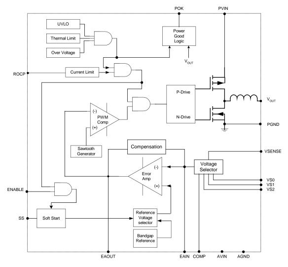
Figure 3. System block diagram.
