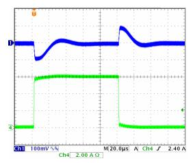
Transient Response  $5.5V_{\text{IN}}/3.3V_{\text{OUT}},$  0-6A, 10A/uS.  $C_{\text{OUT}}$  = 50uF
