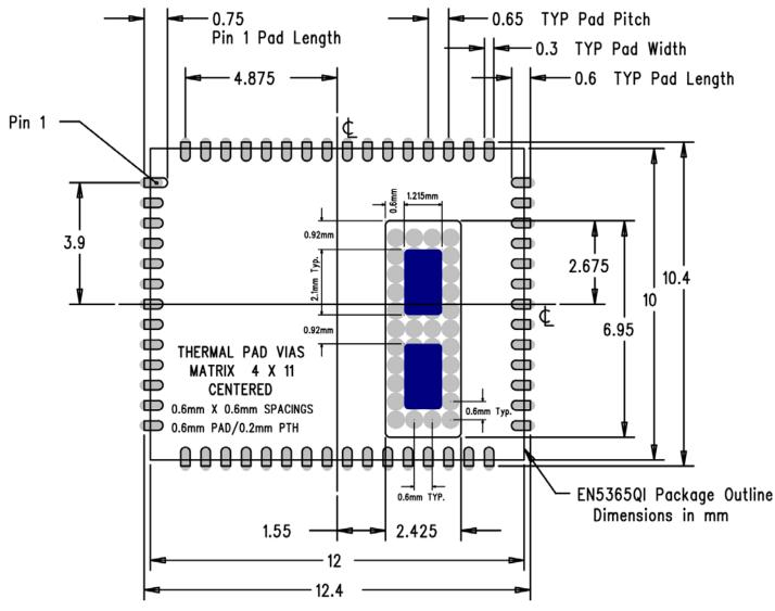
Figure 8: EN5365QI PCB Footprint (Top View)
