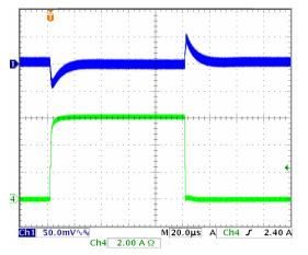
Transient Response  $5.5V_{\text{IN}}/1.2V_{\text{OUT}},$  0-6A, 10A/uS.  $C_{\text{OUT}}$  = 50uF
