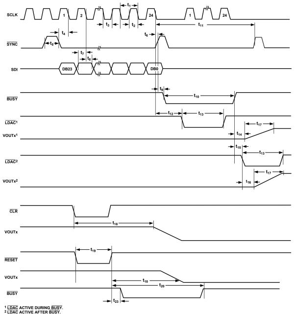
Figure 4. SPI Write Timing
