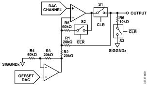
Figure 20. Output Amplifier and Offset DAC
