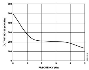
Figure 13. Output Noise Spectral Density
