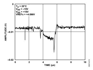
Figure 10. Analog Crosstalk Due to LDAC
