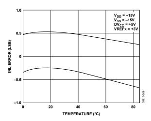
Figure 9. Typical INL Error vs. Temperature
