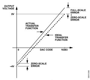
Figure 6. DAC Transfer Function
