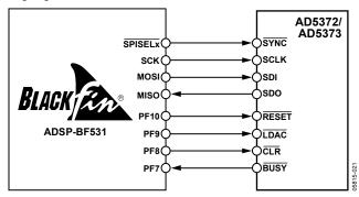
Figure 21. Interfacing to a Blackfin DSP
