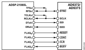
Figure 22. Interfacing to an ADSP-21065L DSP
