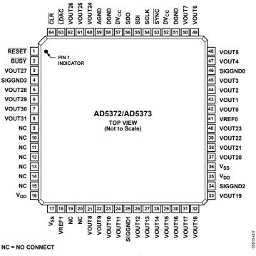
Figure 7. Pin Configuration
