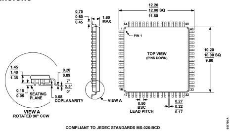
Figure 23. 64-Lead Low Profile Quad Flat Package [LQFP] (ST-64-2) Dimensions shown in millimeters
