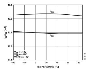
Figure 15.  $I_{DD}/I_{SS}$  vs. Temperature
