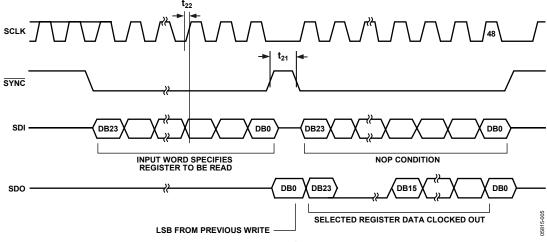
Figure 5. SPI Read Timing
