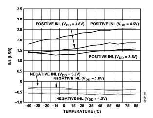
Figure 13. INL vs. Temperature vs. Supply
