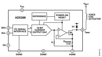
Figure 17. Block Diagram Showing Connection to Voice Coil
