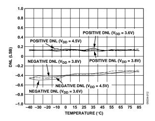
Figure 14. DNL vs. Temperature vs. Supply
