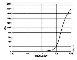
Figure 12. AC Power Supply Rejection ( $V_{DD} = 3.6 V$ )
