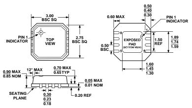
Figure 25. 8-Lead Lead Frame Chip Scale Package [LFCSP\_VD] 3 mm × 3 mm Body, Very Thin, Dual Lead (CP-8-2) Dimensions shown in millimeters
