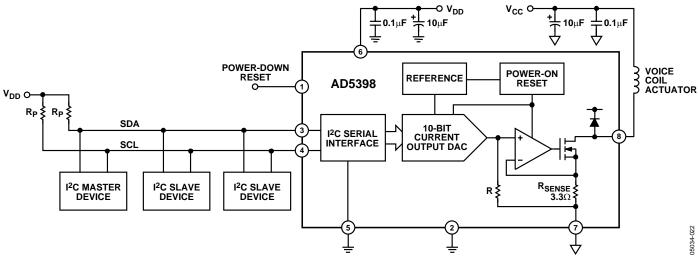
Figure 23. Typical Application Circuit
