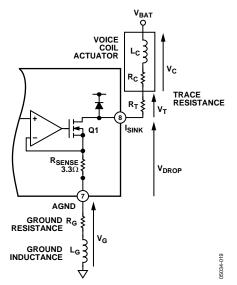
Figure 21. Effect of PCB Trace Resistance and Inductance
