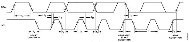
Figure 2. 2-Wire Serial Interface Timing Diagram
