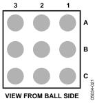
Figure 4. 9-Ball WLCSP Pin Configuration
