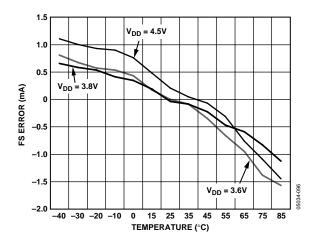
Figure 16. Full-Scale Error vs. Temperature vs. Supply
