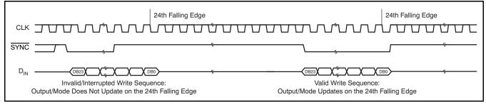
Figure 95. SYNC Interrupt Facility
