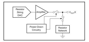
Figure 96. Output Stage During Power-Down
