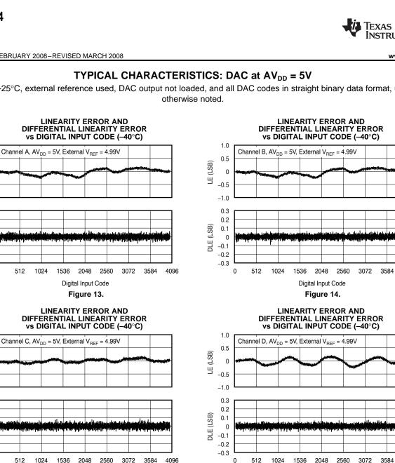
At T<sub>A</sub> = +25°C, external reference used, DAC output not loaded, and all DAC codes in straight binary data format, unless
