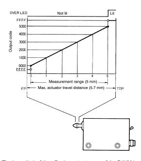
The lower limit of the effective output range of the D5VM in BCD mode is factory-set to 0000.
