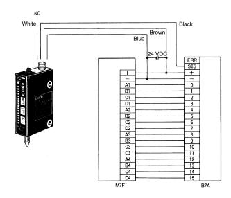
The B7A must be a 16-point output model with a standard transmission delay (i.e., 19.2 ms).
