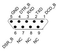
Figure 3-2 SCI Connector J53 Pin Assignments
