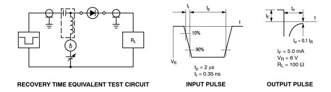
Figure 4. Reverse Recovery Time Test Circuit for the DAN222
