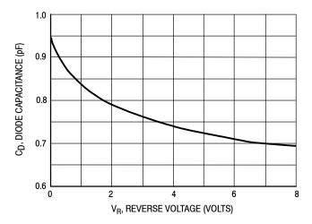
Figure 3. Diode Capacitance
