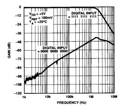
Gain vs. Frequency (Output Amplifier: OP42)
