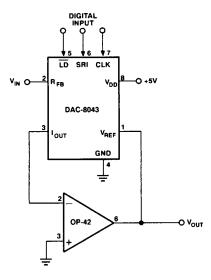
Figure 8. Analog/Digital Divider
