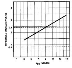
Logic Threshold Voltage vs. Supply Voltage
