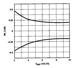
Linearity Error vs. Reference Voltage
