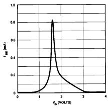
Supply Current vs. Logic Input Voltage
