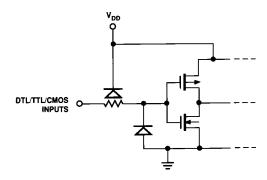
Figure 1. Digital Input Protection
