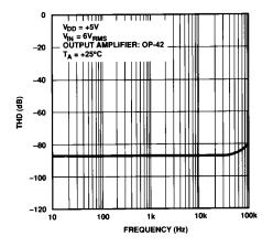
Total Harmonic Distortion vs. Frequency (Multiplying Mode)
