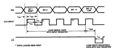
Write Cycle Timing Diagram
