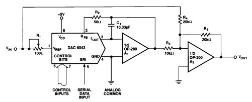
Figure 7. Bipolar Operation (4-Quadrant, Offset Binary)
