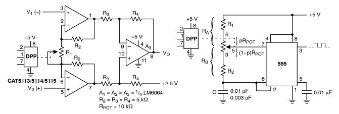
Figure 7. Programmable Instrumentation Amplifier
