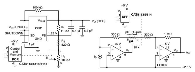
Figure 10. Programmable Voltage Regulator
