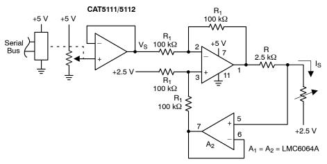
Figure 14. Programmable Current Source/Sink
