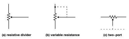
Figure 6. Potentiometer Configuration
