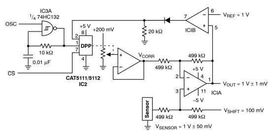
Figure 9. Sensor Auto Referencing Circuit
