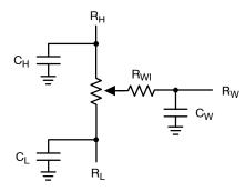
Figure 4. Potentiometer Equivalent Circuit
