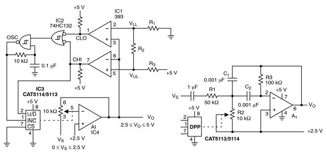
Figure 12. Automatic Gain Control
