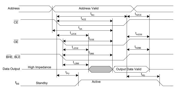
Figure 7. SRAM Read Cycle #2:  $\overline{\text{CE}}$  and  $\overline{\text{OE}}$  Controlled [3, 14, 18]
