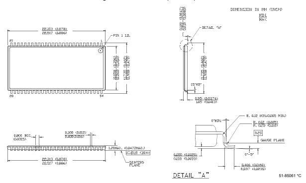
Figure 18. 32-Pin SOIC (51-85127)
