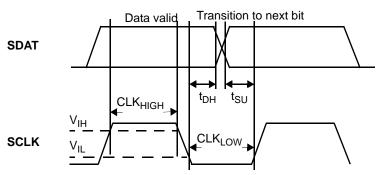
Figure 4. Data Frame Architecture
