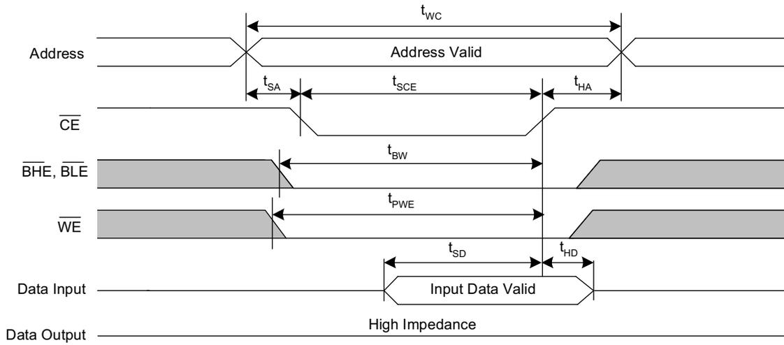
Figure 10. SRAM Write Cycle #3:  $\overline{BHE}$  and  $\overline{BLE}$  Controlled [3, 17, 18, 19]
