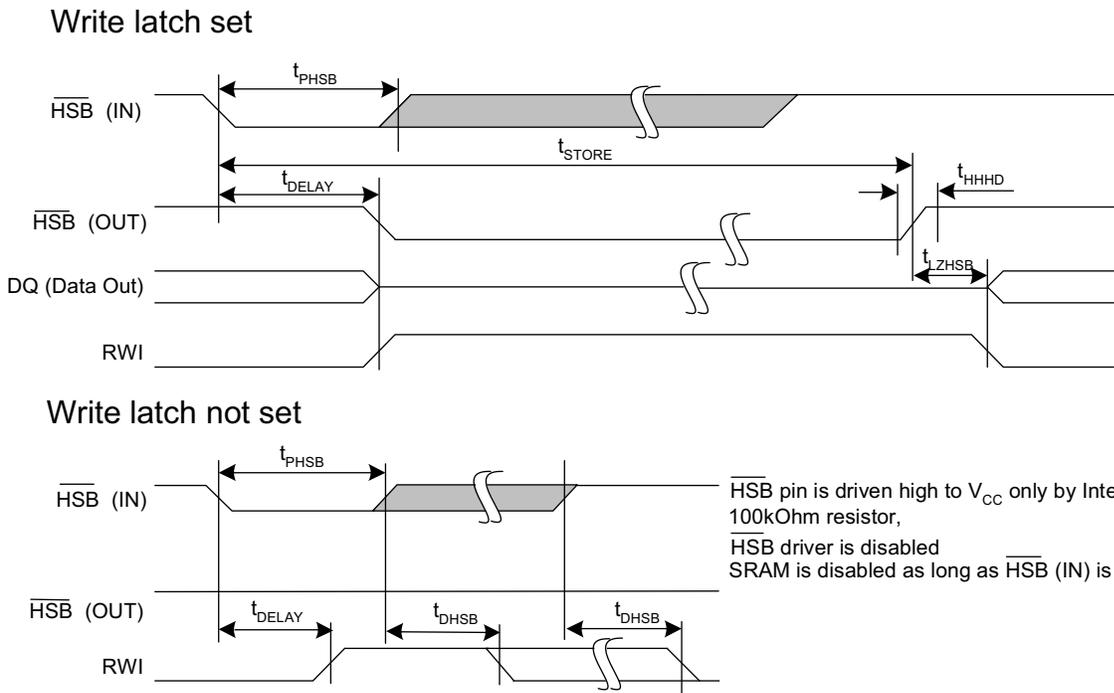
Figure 15. Soft Sequence Processing<sup>[28, 29]</sup>
