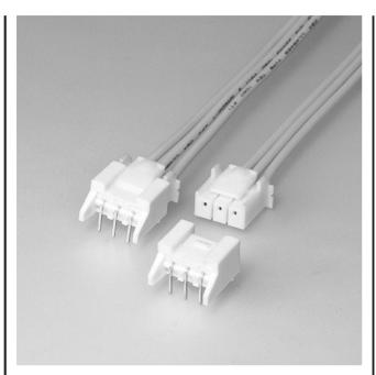
VU connector is small type 3.96mm pitch PC board connector for large current and has the high reliability in a power supply circuit, considering the fully shrouded connector header structure against "vibrating connector" and "distorted extraction".
