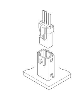
This JWPF connector can be used for the place of which especially waterproof is reauired.
