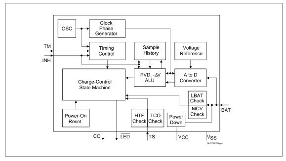
Figure 3. Block Diagram
