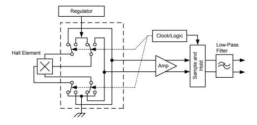
Figure 2. Model of chopper stabilization technique
