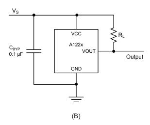
Figure 1. Switching behavior of latches. In panel A, on the horizontal axis, the B+ direction indicates increasing south polarity magnetic field strength, and the B- direction indicates decreasing south polarity field strength (including the case of increasing north polarity). This behavior can be exhibited when using a circuit such as that shown in panel B.
