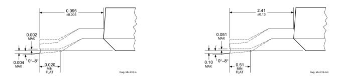
NOTES: 1. Tolerances on package height and width represent allowable mold offsets. Dimensions given are measured at the widest point (parting line).
