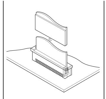
The FMZ series, a Zero Insertion Force (ZIF) connector series, was developed to increase wear resistance and extend the connector's mating life. It is a very compact connector with a thickness of only 4.2 mm and a pitch of only 1.0 mm and is thus useful for high density packaging. The contact has a reliable double-leaf construction which provides stable connection.
