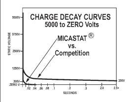
The premium choice for ESD bench dissipative worksurfaces. Provides a durable and attractive ESD controlled dissipative worksurface. Resists hot solder and most solvents; exceeds NEMA standards for wear resistance. Patented conductive layer provides superior charge dissipation and zero voltage suppression.
