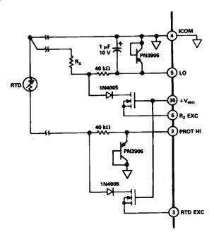
Figure 3. 120 V/240 V AC Normal Mode Input Protection
