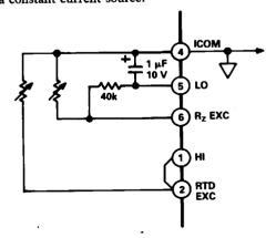
Figure 4. Differential RTD Measurement
