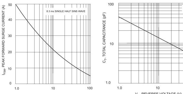
NUMBER OF CYCLES AT 60Hz Fig. 3 Maximum Non-Repetitive Peak Forward Surge Current
